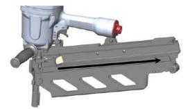
**Open the magazine:** Pull pusher back to engage the latch.
