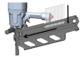
**Nail loading:** Hold nailer down with magazine tilted downward. Insert stick of nails.
