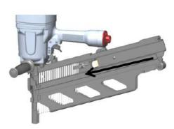
**Close Magazine:** Release push by pressing latch Slide pusher against nails.
