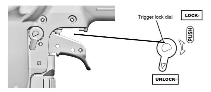
The tool is equipped with a Trigger Lock mechanism. Push and rotate the Trigger Lock Dial to the trigger free position before driving nails.
