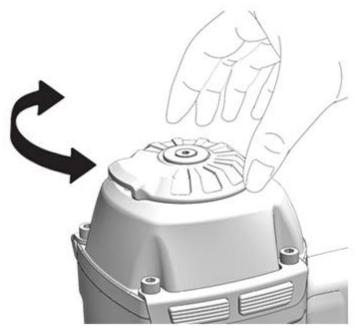
exhaust air is changed by cover by hand,
